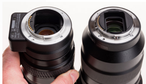
With the E-mount flange in the same position, note how far from the sensor the old DSLR 24-105mm rear element is placed, and how close the rear glass of the FE design can be with the 18mm register. It's this freedom to rethink optical design which has enabled a 24-105mm with near-prime performance (at a price).
